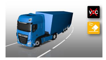
In case of understeer the front of the vehicle slides to the outside edge of the curve and if uncorrected, will leave the road. VSC will apply the brakes at the curve-inside wheels to bring the tractor back on its intended path.
